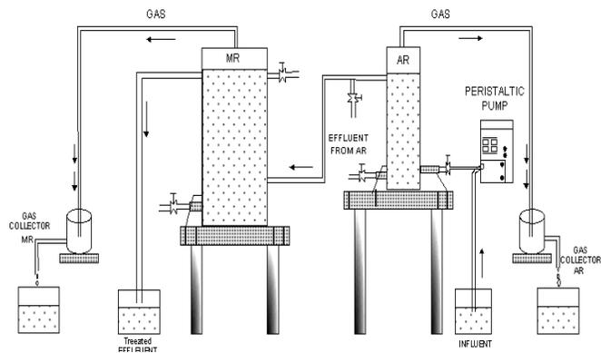
**Fig. 1 Schematic diagram of the diphasic digester**
